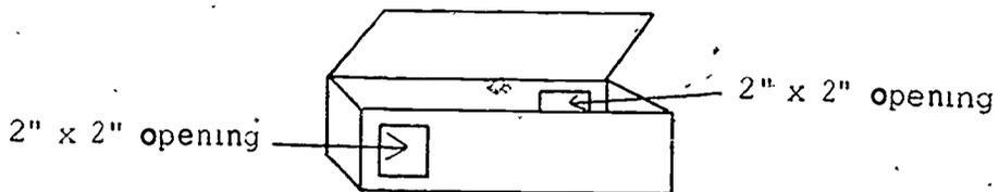
Make a  $2\frac{1}{4}$ " slit on each side as shown in the diagram below. The slits should be approximately  $2\frac{1}{4}$ " from the corners on the long sides and  $\frac{1}{2}$ " from the corners on the short sides.
