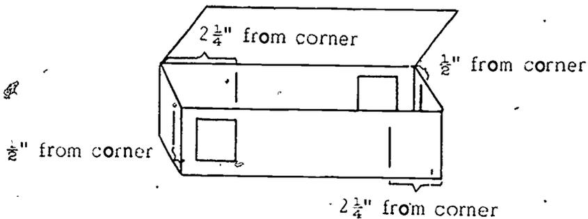
Small mirrors can be placed in the corners opposite each opening by fitting them into the slits.
