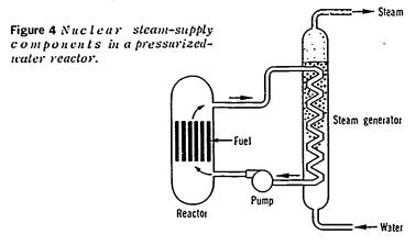
As you can see, a nuclear steam supply that uses a pressurized-water reactor consists of two separate water systems that meet in the steam generator. The water in one system does not mix with that in the other, but heat is transferred from the reactor system to the steam system.
