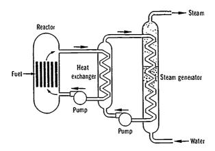
Figure 7 Nuclear steam-supply components in a liquid-metal-cooled breeder reactor.
