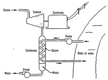
Figure 2 The power-generating portion of a nuclear power plant.
