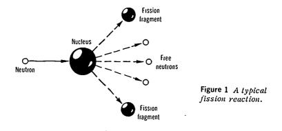
Sustaining the chain reaction is important because more than 30 billion fissions must occur in one second to release each watt of energy. If the chain reaction is to be useful, the fissions must occur at a desired rate, and the heat that is generated by the process must be removed. The job of the nuclear reactor, then, is to provide an environment in which fission reactions can be initiated, sustained, and controlled, and to make possible recovery of the resultant heat.\*
