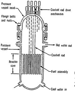
Figure 9 Vertical cross section view of a pressurized-water reactor vessel.
