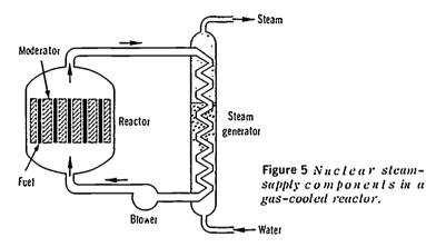
because the cooling water serves this purpose. Gas isn't a very good moderator, however, so in gas-cooled reactors a special material, usually graphite, is built in.
