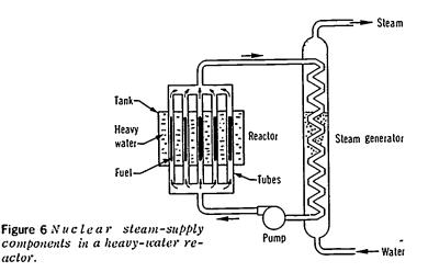
Any of several cooling fluids — organic compounds, gas, water. or heavy water — can be used in heavy-water reactors, since the heavy-water moderator is separated from the cooling fluid by the walls of the process tubes.
