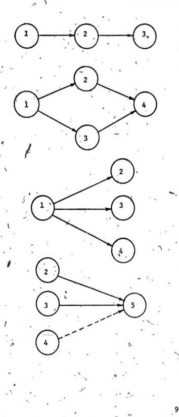
SERIES Construction-a linear progressive chain is developed. Event 1 must be completed before event 2 and event 2 must be completed before event 3.
