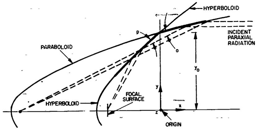
Figure 8. Two reflections from a paraboloid and hyperboloid of resolution.
