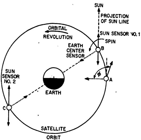
Figure 6. Determination of satellite position.
