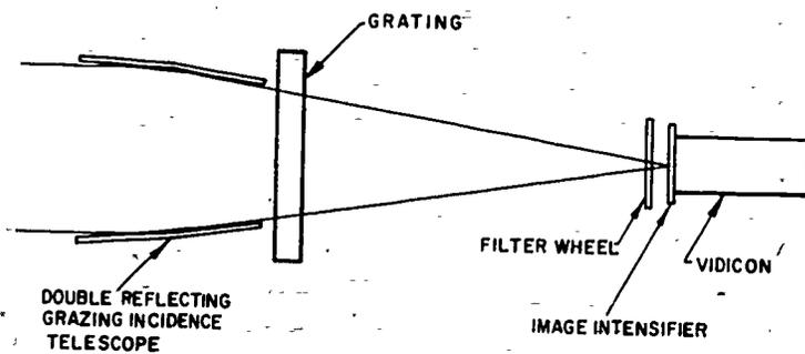
Figure 7. New method for solar X-ray studies.
