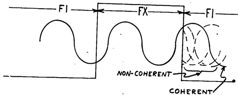
Figure 2. Phase coherent frequency switching.
