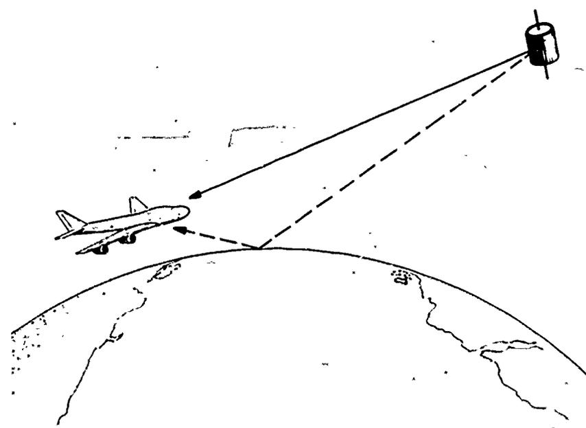
Figure 9. Multipath propagation.
