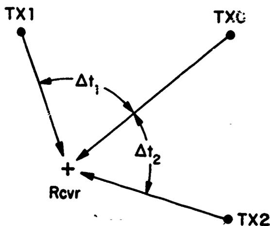
Figure 17. Radio generation of reference hyperbolas for position finding.
