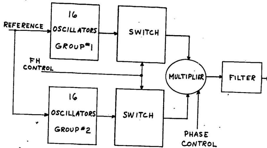
Figure 3. Simplified block diagram of the Phase Coherent Frequency Synthesizer.
