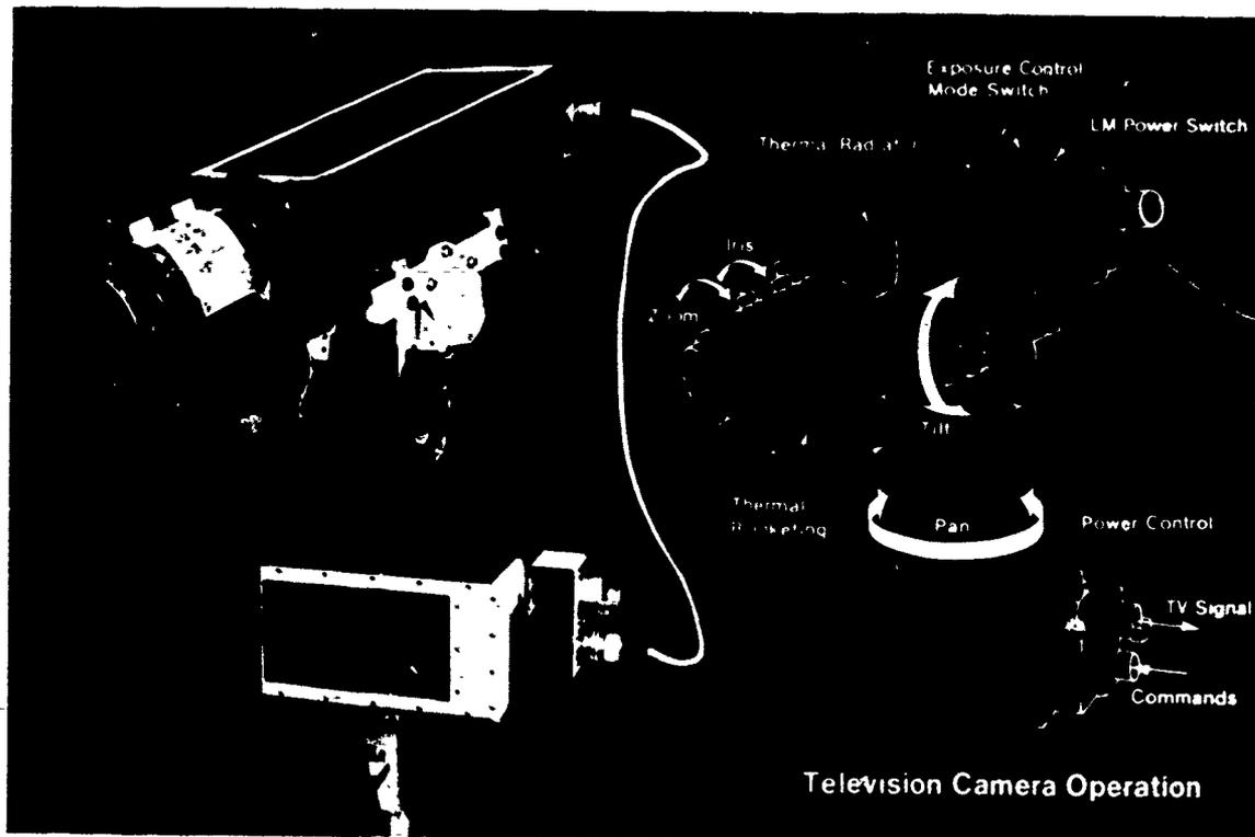
Figure 3. Ground Commanded Television Assembly (GCTA).
