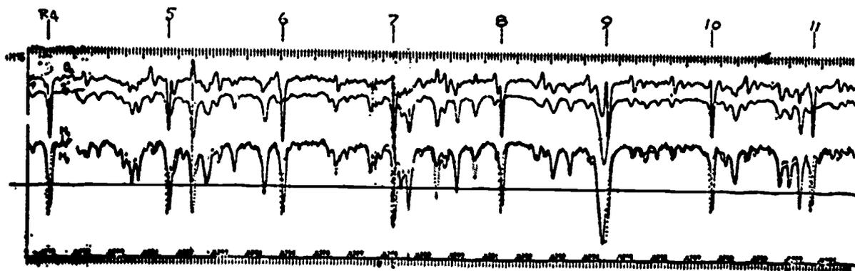
Figure 18. Solar spectrum showing 2-0 band of CO ( $S_A$  is the solar spectrum; the marks show the CO line positions).
