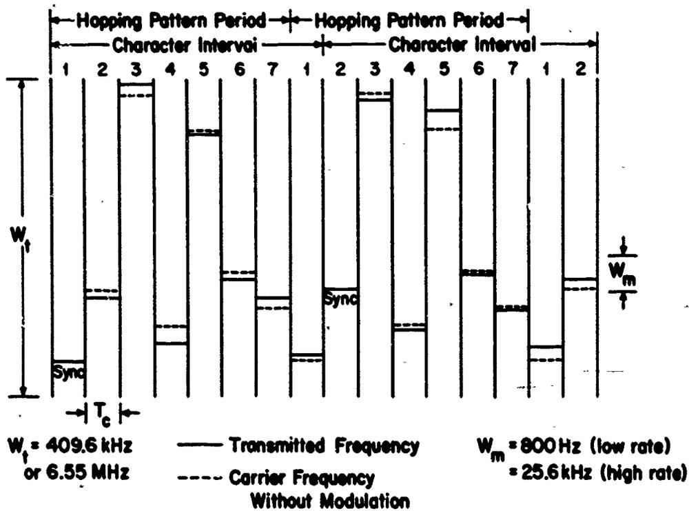
Figure-14. TATS bandspread signal format-fixed pattern.
