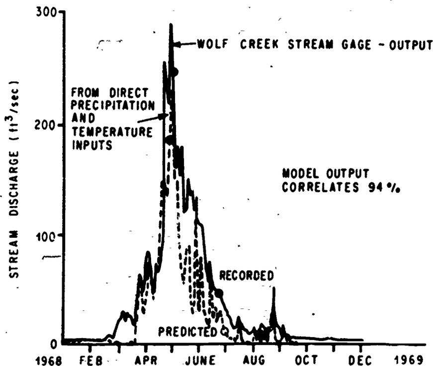
Figure 6. Records used for establishing hydrological model of Wolf Creek Drainage Basin.
