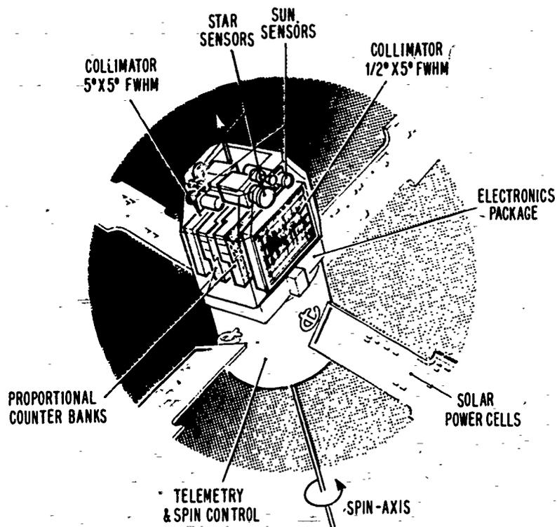
Figure 4. Uhuru's fields of view and scanning mode.
