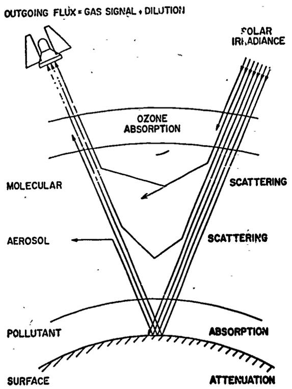
Figure 2. Attenuation and dilution in the ultraviolet.
