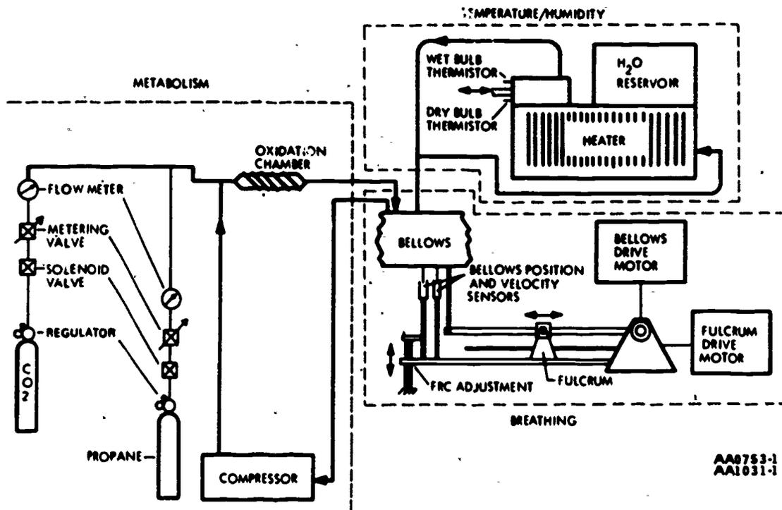
Figure 1. BMS subsystems.
