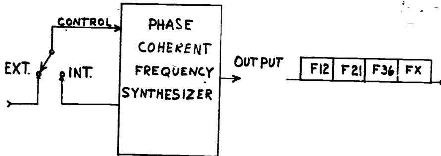
Figure 1. Phase Coherent Frequency Synthesizer, simplified.
