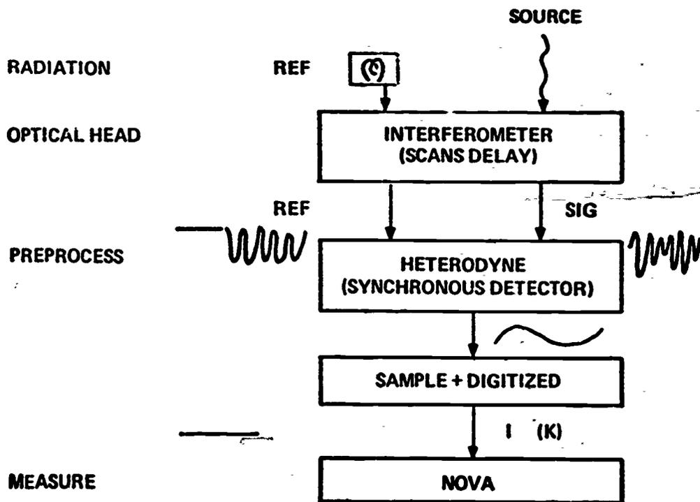
Figure 22. Interferometer system block diagram.
