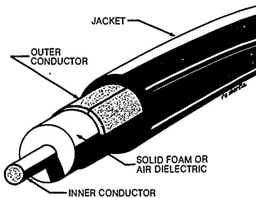
apart and maintains an electric field between them. An outer plastic sheath protects the cable from weather or whatever else might affect the system's operation.
