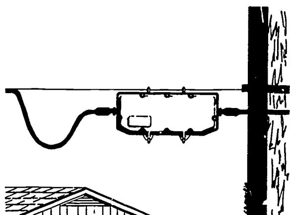
Performance standards limit the number of amplifiers that can be connected in line on one coaxial cable to about 25 trunk amplifiers, spaced 2.8 amplifiers per mile of 3/4-inch cable. This rule of thumb implies that trunk lines cannot extend more than approximately eight miles from each headend without unacceptable loss of signal quality.
