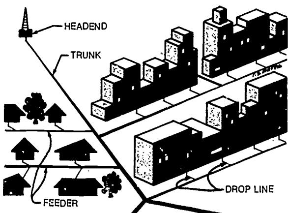
The cable that leaves the headend, called the trunk line, is about one-half to three-quarters of an inch in diameter. To distribute the cable to subscribers' homes, the trunk line is connected to smaller feeder lines. Finally, individual drop lines run into each household.
