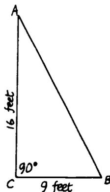
In the above diagram, AB is a ladder leaning against a wall. What is the length of the ladder? ( $AB^2 = AC^2 + BC^2$ )
