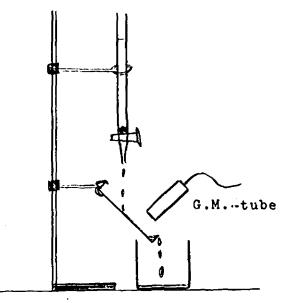
Fig. 6 Ion exchange set-up
