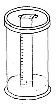
Fig. 5 Paper chromatographic set-up
