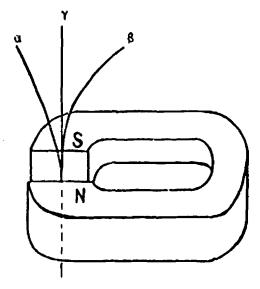
Fig. 3 Deflection of radiations by magnetic field
