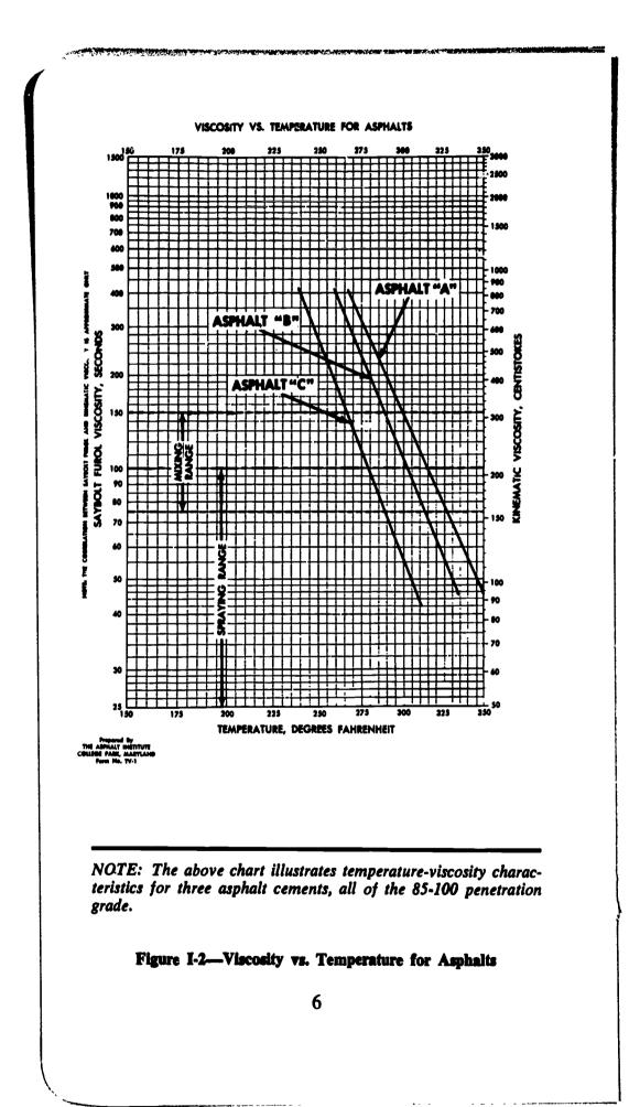
ERIC Full Box Provided by ERIC data should be available at the plant at all times to aid in determining the proper temperature of the completed batch. Using the viscosity information, the engineer should designate the temperature of the completed mix at the plant and at the paver. Since the bulk of any mix is the aggregate, the temperature at which it is introduced into the mixer controls the mixing temperatures.
