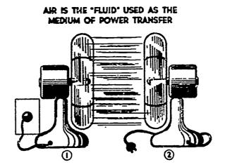
Fig. 2 Simple fluid coupling (air serving as fluid)
