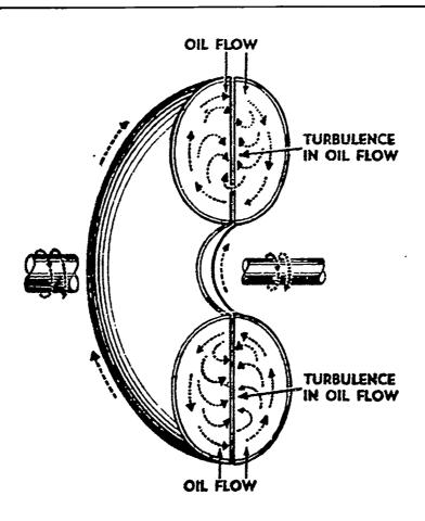
Plate II Turbulence in oil flow within the fluid coupling
