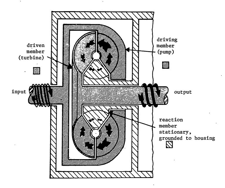
Plate IV Torque converter schematic
