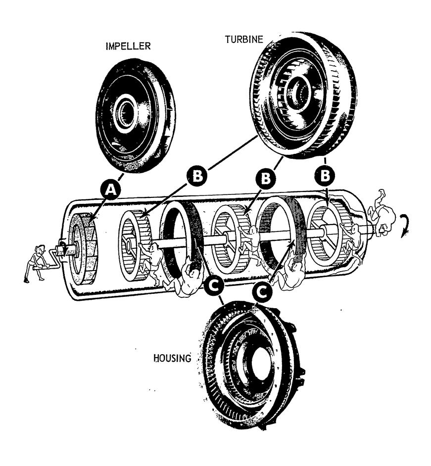
Fig. 18 Operation of a three stage torque converter
