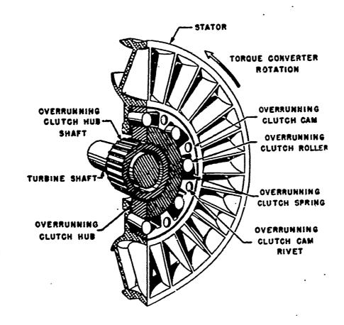
Fig. 12 Roller type stator
