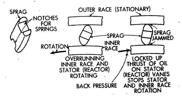
Fig. 13 Appearance and action of a sprag
