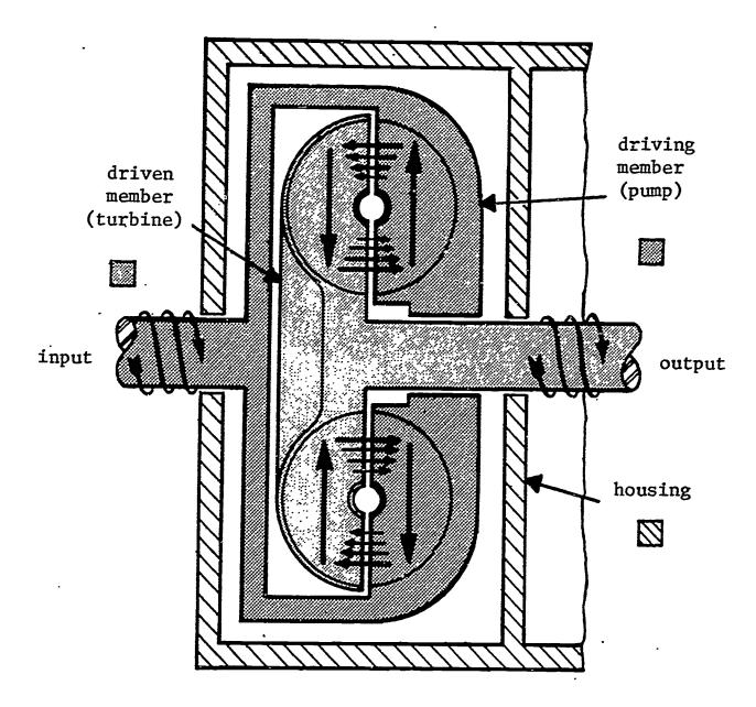
Plate III Fluid coupling schematic
