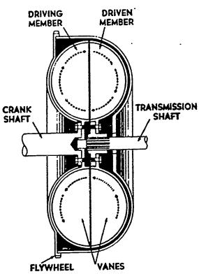
Fig. 1 Cross sectional view of a fluid coupling
