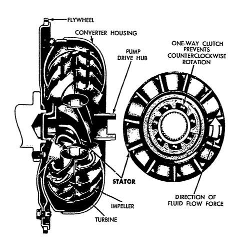
Fig. 14 Converter in torque multiplication phase
