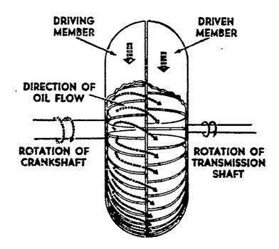
Plate I Fluid coupling in action
