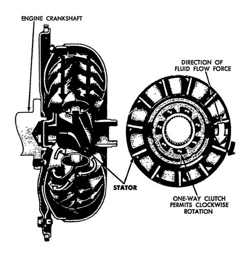
Fig. 15 Converter in fluid coupling phase
