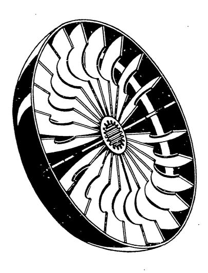
Fig. 3 Fluid coupling pump
