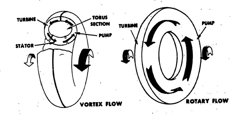
Fig. 11 Oil flow within a converter
