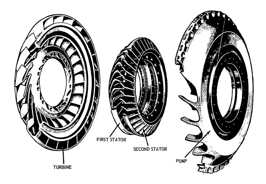
Fig. 16 Four element torquatic converter
