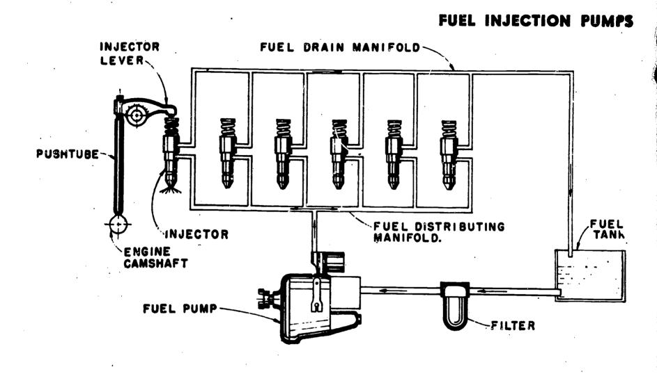
Fig. 2 Cummins fuel arrangement.
