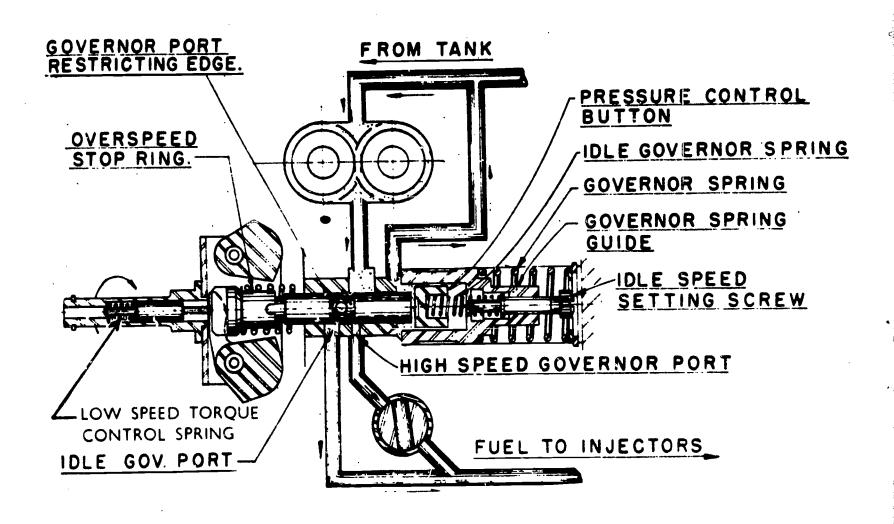
Fig. 5 Schematic flow diagram of Cummins fuel pump.
